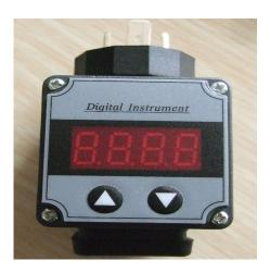
Common two-wire loop-powered led display for all two-wire transmitters, such as: pressure, differential pressure, temperature, flow, pH value, acceleration and Force, etc. Its microprocessor based, two key programming, achieve zero, full scale, decimal point, display rate
